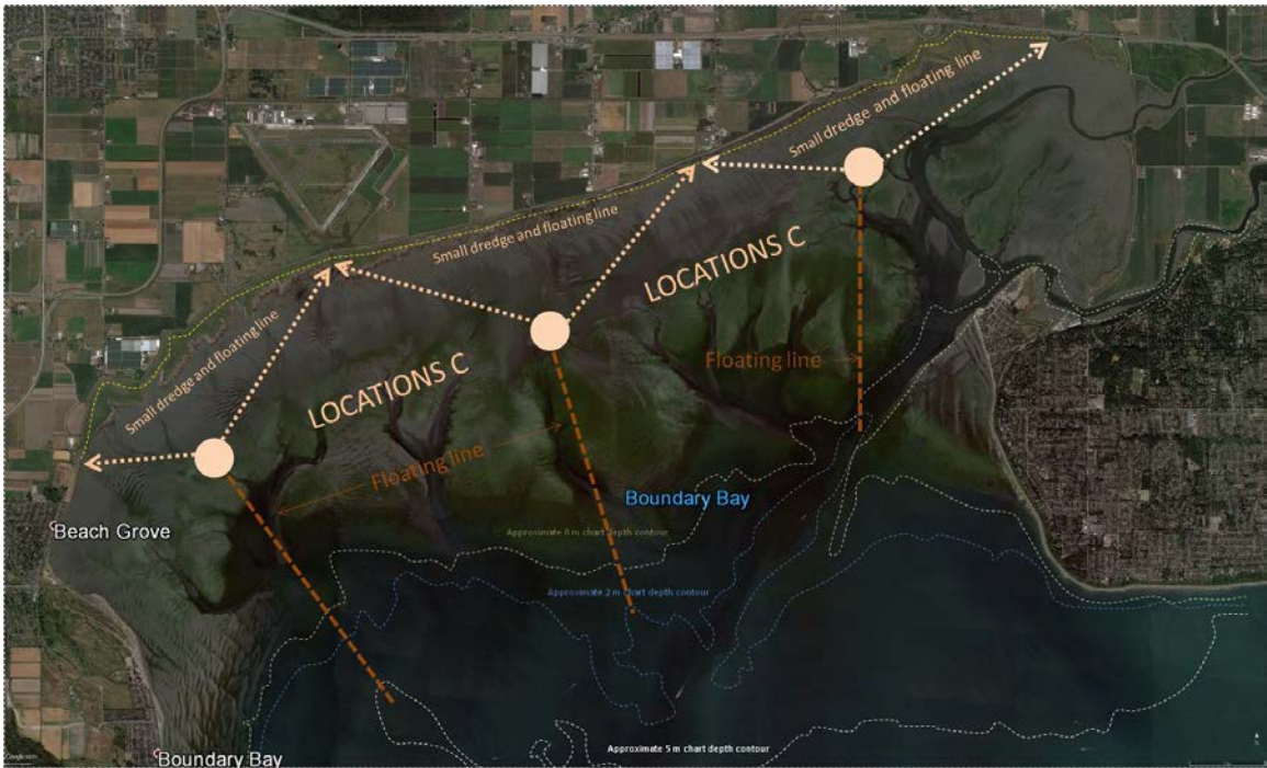
Figure 15: Sand Delivery System for Method C
