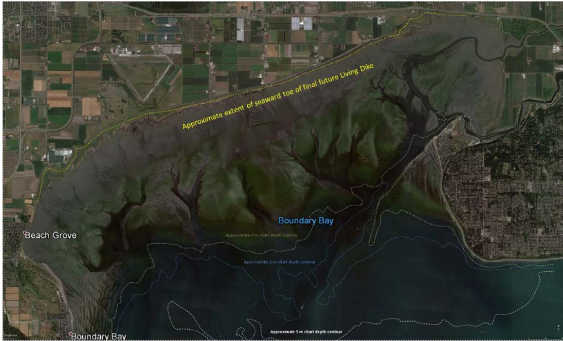
Figure 12: Approximate Location of seaward toe of final Living Dike (note: Canada - US border is at bottom of image) (contours shown are from CHS chart 3463)
